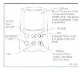
Fig.7 Transmitter diagram
